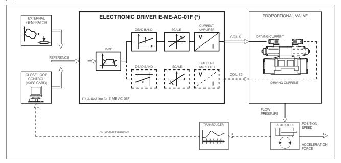
E-ME-AC drivers control the current to the solenoid of Atos proportional valves without pressure or position transducer, regulating the spool position, the flow or the pressure according to the electronic reference signal.
